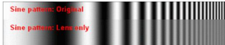
Sine wave response. Upper: input, Lower: blurred output
