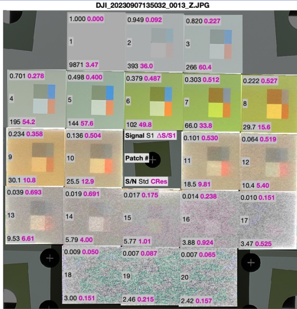
8000x6000 pixels uint8 gamma = 0.443 Constant xyY mean patch = 99x143px
